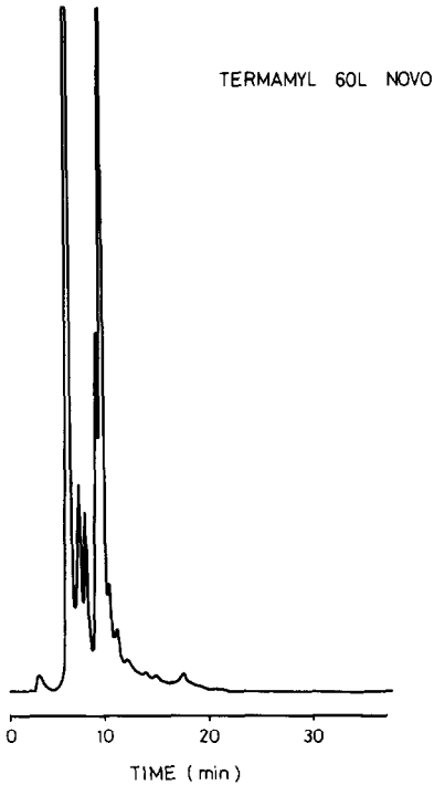
Fig. 7. Chromatogram of Termamyl 60 L industrial enzyme. Conditions as in Fig. 5.
